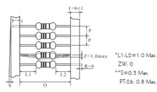
Dimension of T/B (mm) 0 P A±5 B±5 C±5 Qty./Box Type 5±0.3 FRN 1/4W  $52\pm1$ 75 116 255 5,000 PCS 52±1 5±0.3 75 116 255 5,000 PCS FRN 1/2WS 52±1 5±0.3 75 116 255 5,000 PCS FRN 0.4W 75 255  $52\pm1$  $5\pm0.3$ 45 1,000 PCS FRN 1/2W 52±1  $5\pm0.3$ 80 70 255 1,000 PCS FRN 3/4W 52±1 5±0.3 80 70 255 1,000 PCS FRN 1W FRN 1.5W  $52\pm1$  $5\pm0.3$ 86 82 255 1,000 PCS 52±1 5±0.3 86 82 255 1,000 PCS FRN 2W  $64\pm5$  $10\pm0.5$ 90 119 255 1,000 PCS FRN 3W
