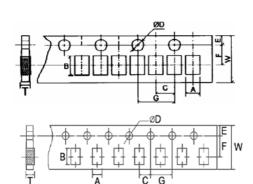
14.2 Dimension of plastic taping: (Unit: mm)
