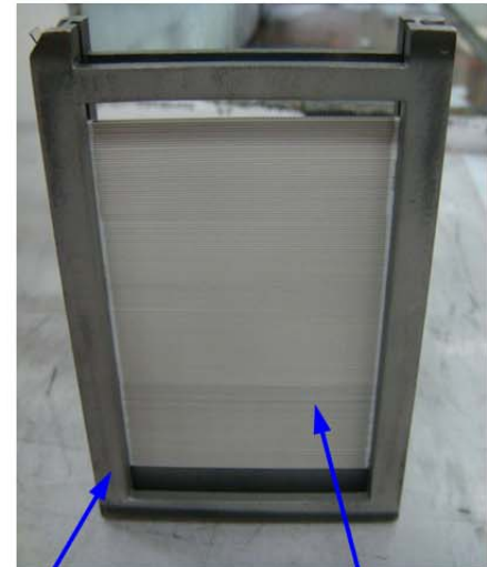
条状半成品堆叠，在仓夹中溅射侧电极 Strips are stacked in cartridge for sputtering
