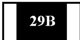
$1.96\text{K}\Omega = 196 \times 10^1\Omega = 29\text{B}$
